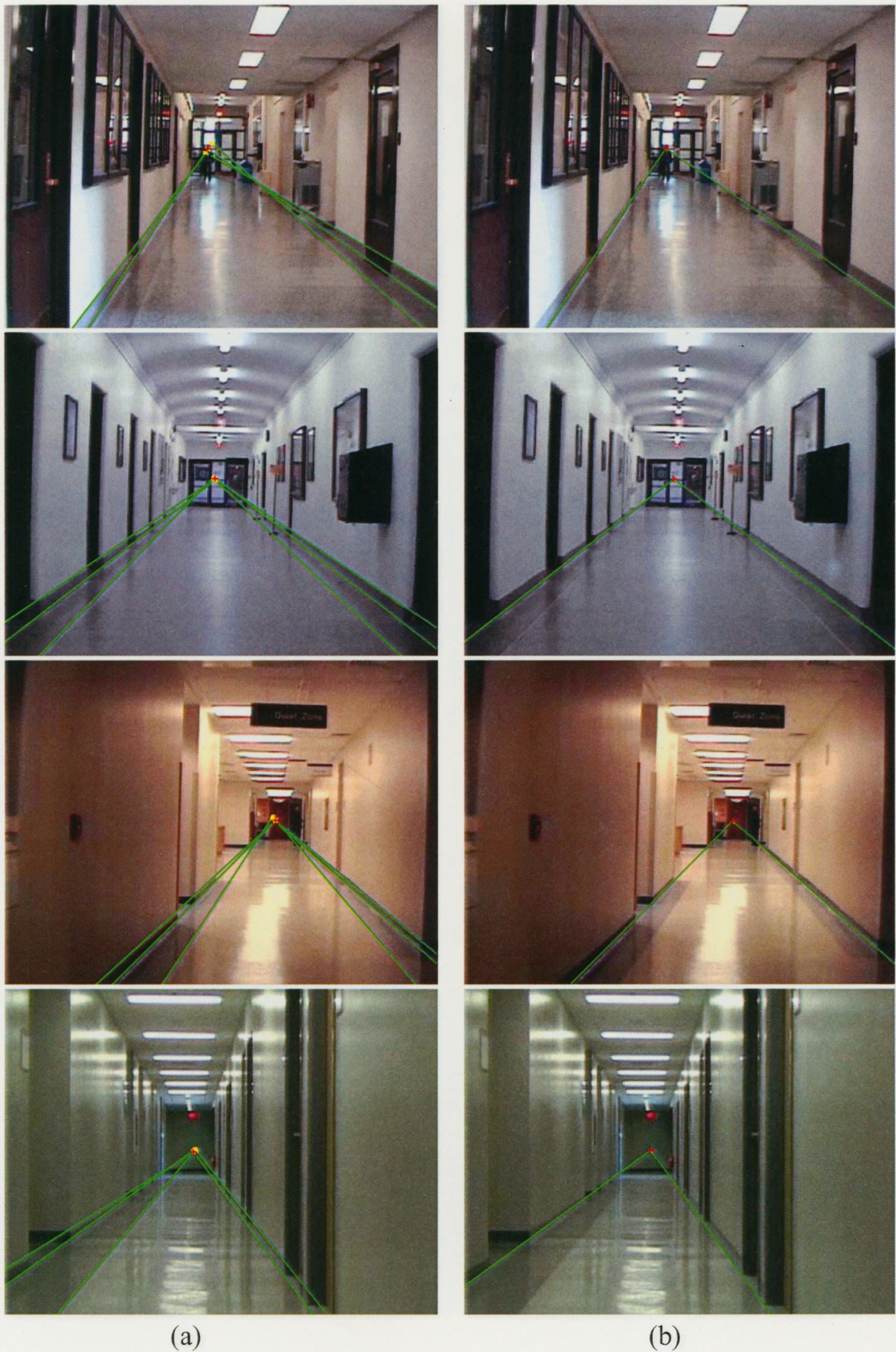
Figure 5.3: Vanishing point and corridor line detecting results (a) Detected vanishing point and generated corridor line hypotheses (b) Detected corridor line locations.
