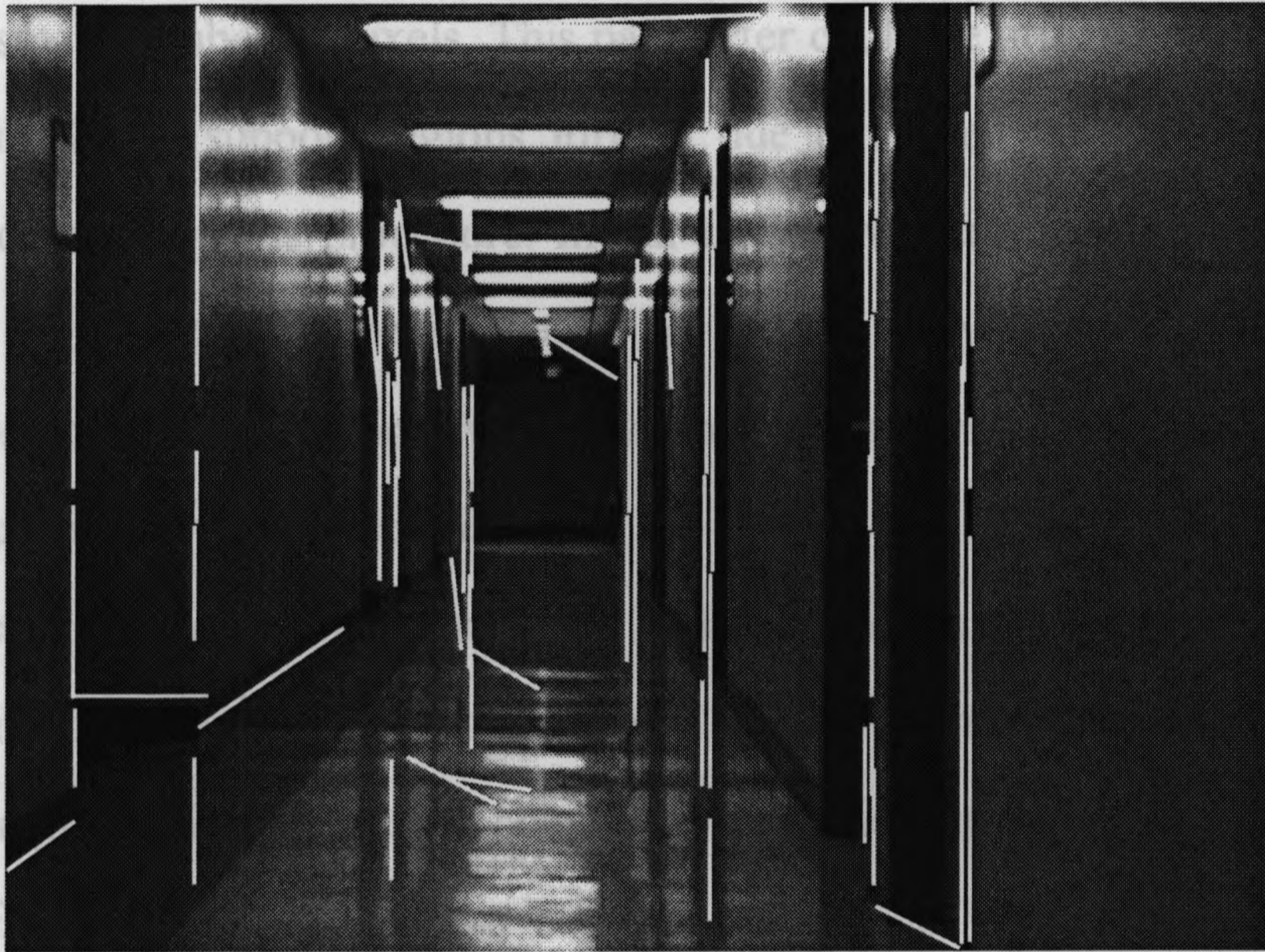
Figure 3.4: Result of applying the standard Hough transform
