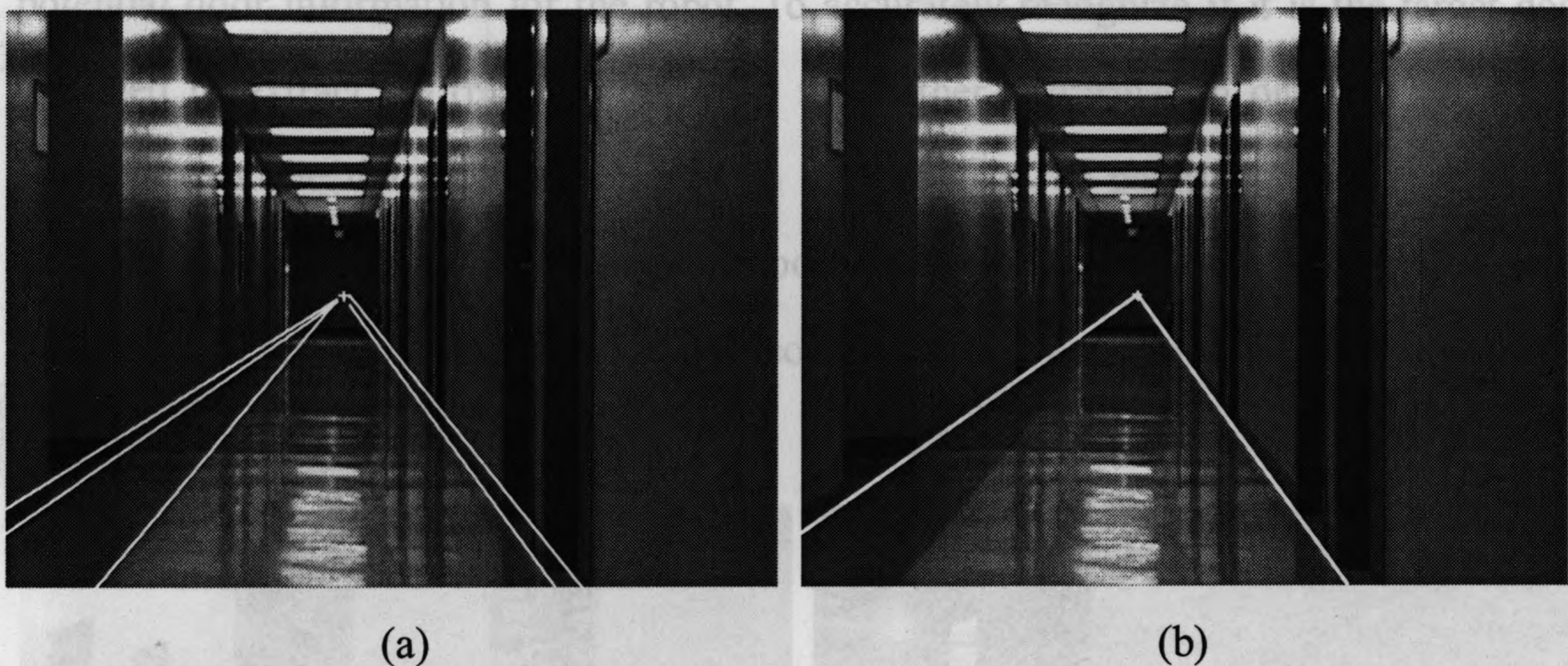
Figure 1.2 Corridor line location detection results (a) Generated corridor line hypotheses and detected vanishing point (b) Detected corridor lines.
