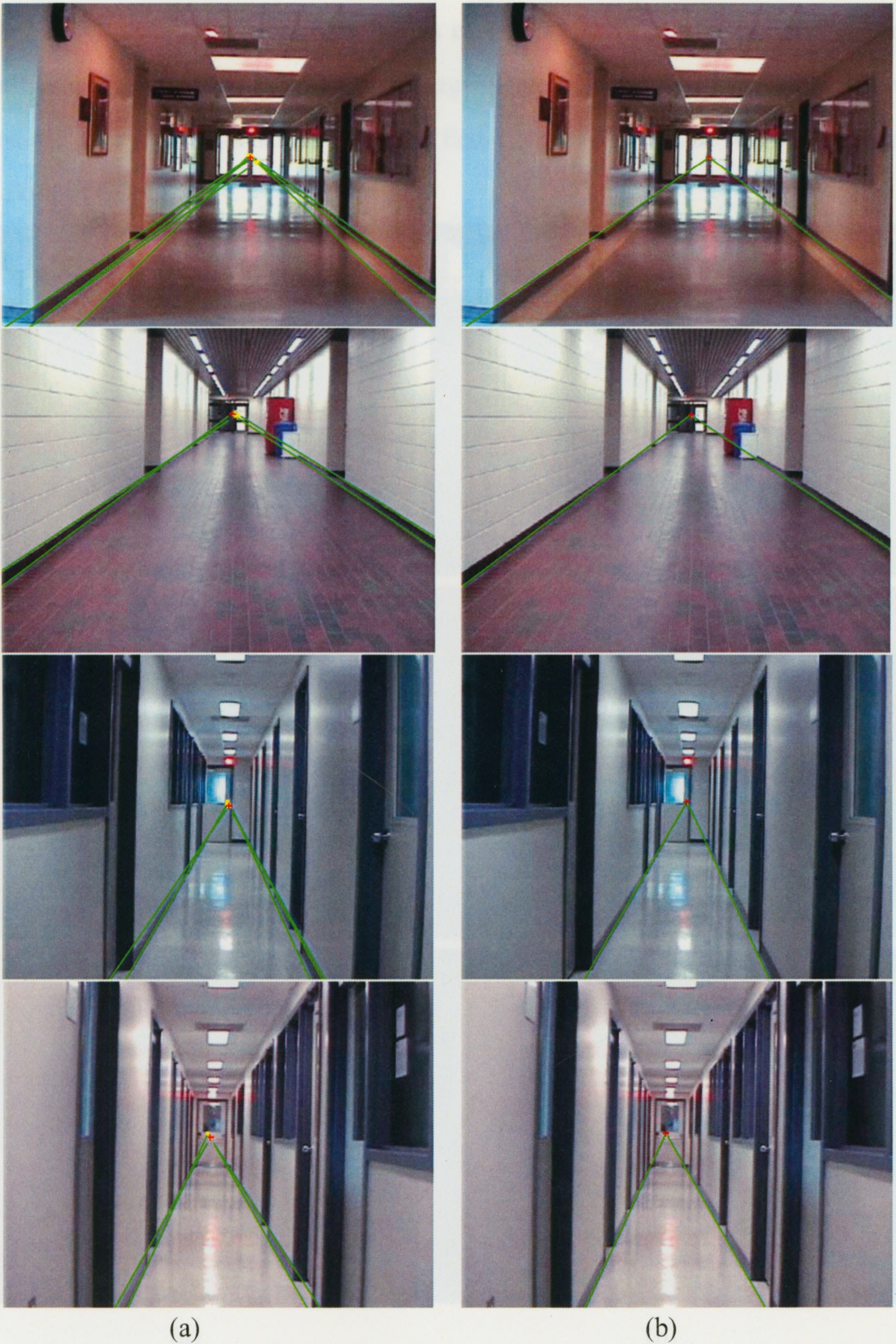
Figure 5.4: Detecting results of corridors with different width: wide corridors in the first two images and narrow corridors in the last two images (a) Detected vanishing point and generated corridor line hypotheses (b) Detected corridor line locations.
