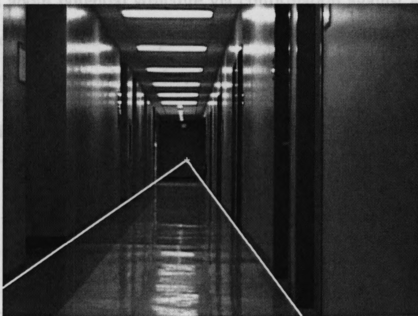
Figure 4.17: Detected corridor lines and the vanishing point
