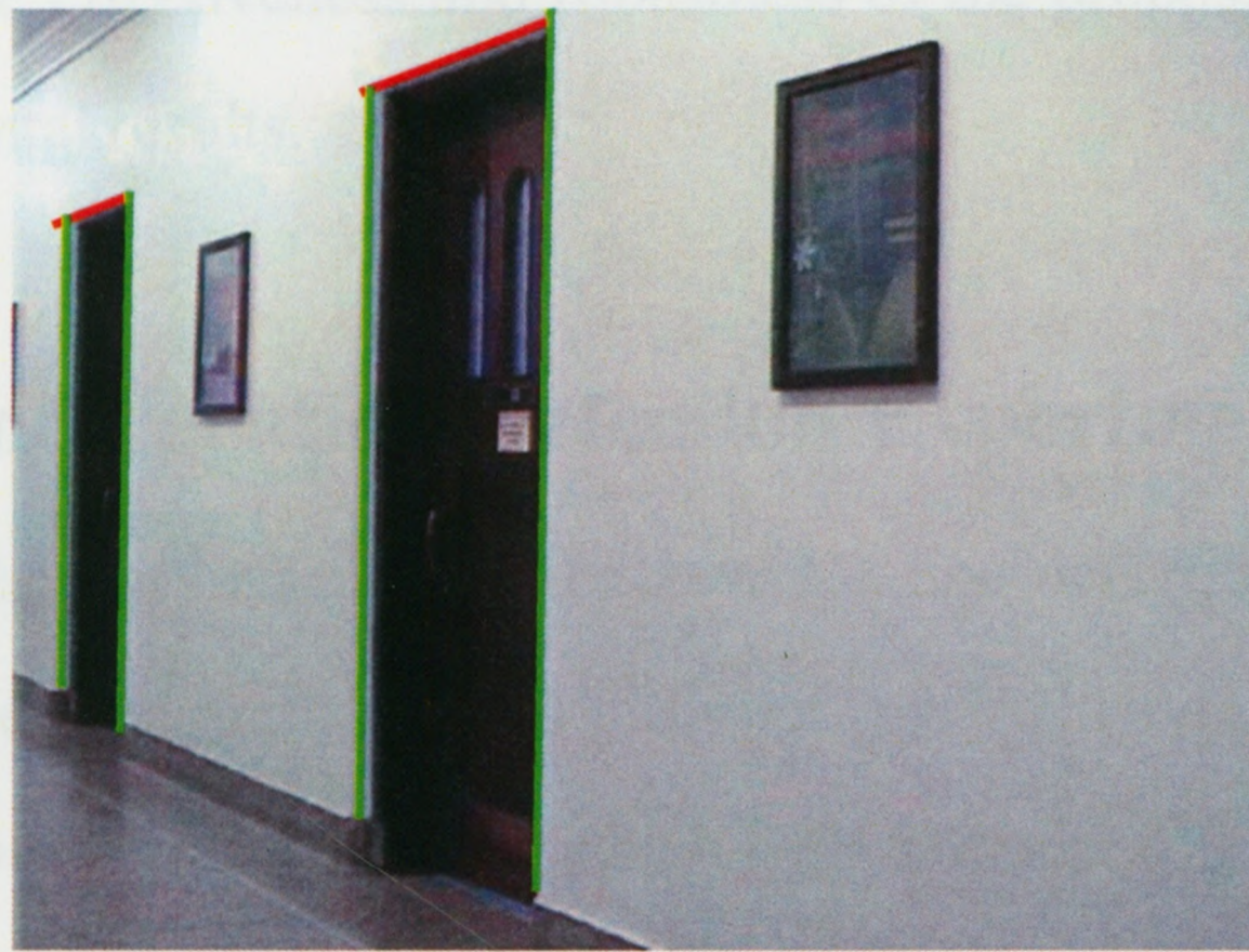
Figure 4.26: Door detection results. Objects similar to door structures such as paintings and posters on the wall are rejected at hypothesis verification stage.
