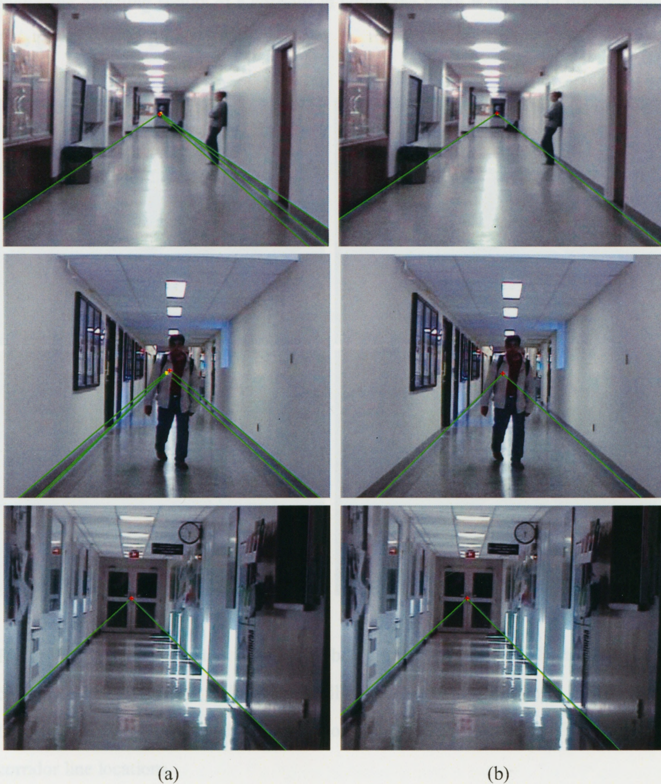
Figure 5.5: Detecting results in the presence of people and strong reflections (the last one) (a) Detected vanishing point and generated corridor line hypotheses (b) Detected corridor line locations
