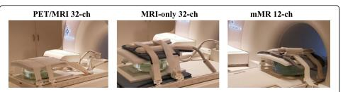
**Fig. 1** Phantom experiment setup for the three arrays PET/MRI 32-channel, MRI-only 32-channel, and mMR 12-channel. Position of isocenter were kept unchanged from one acquisition to the other
