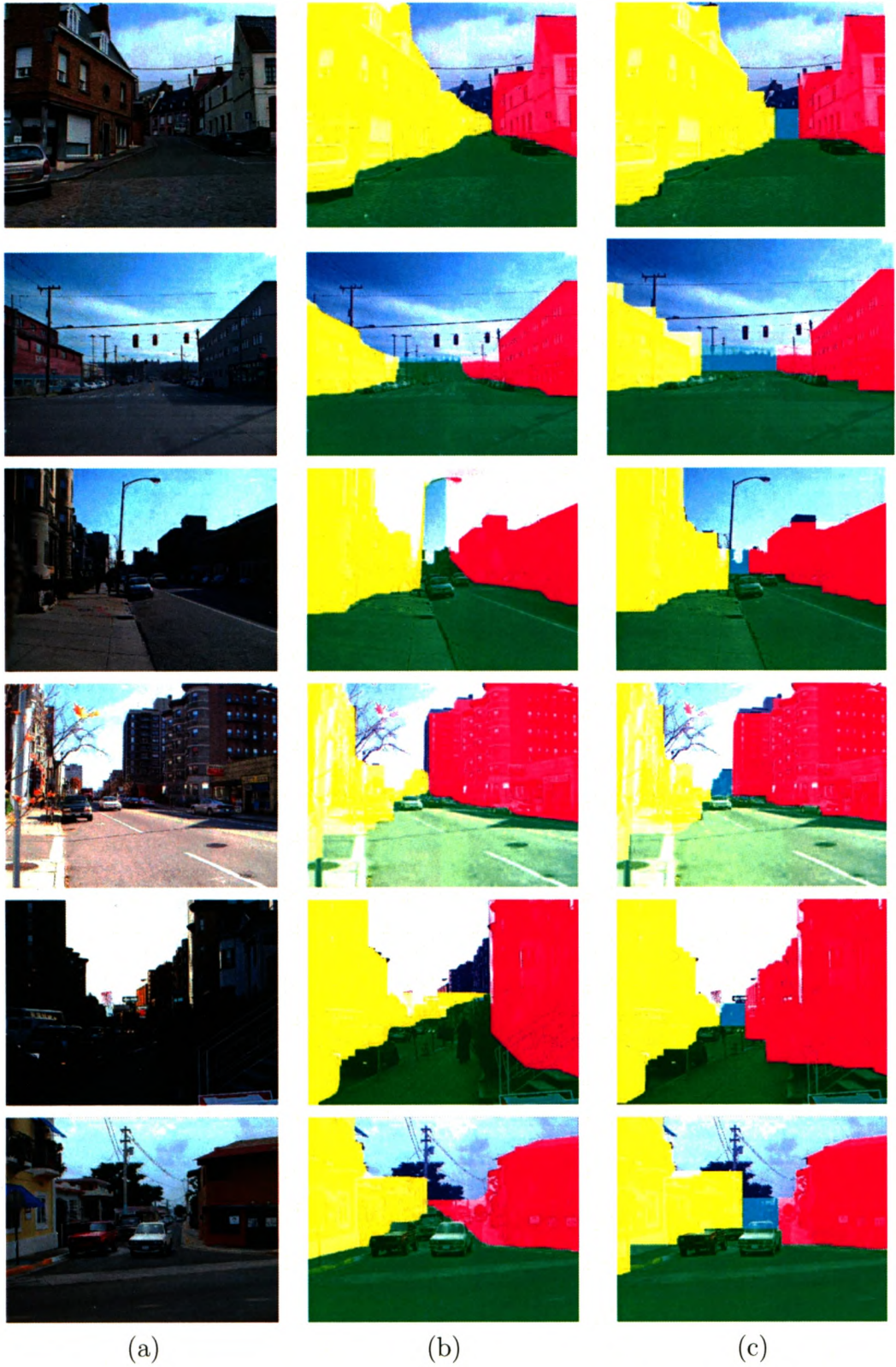
Figure 5.7: Outdoor image result comparison: (a) original images, (b) \alpha -expansion with ordering constraints, (c) order-preserving moves.
