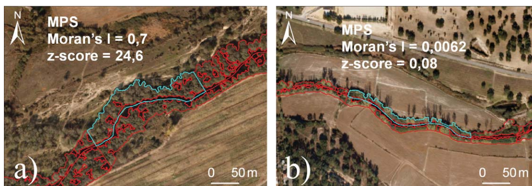
Fig. 7. Morans' I and z-score for the Mean Patch Size (MPS) for the tree cover class. Illustration of: (a) high spatial dependence (River Sôr); and (b) spatial independence (River Muge).
