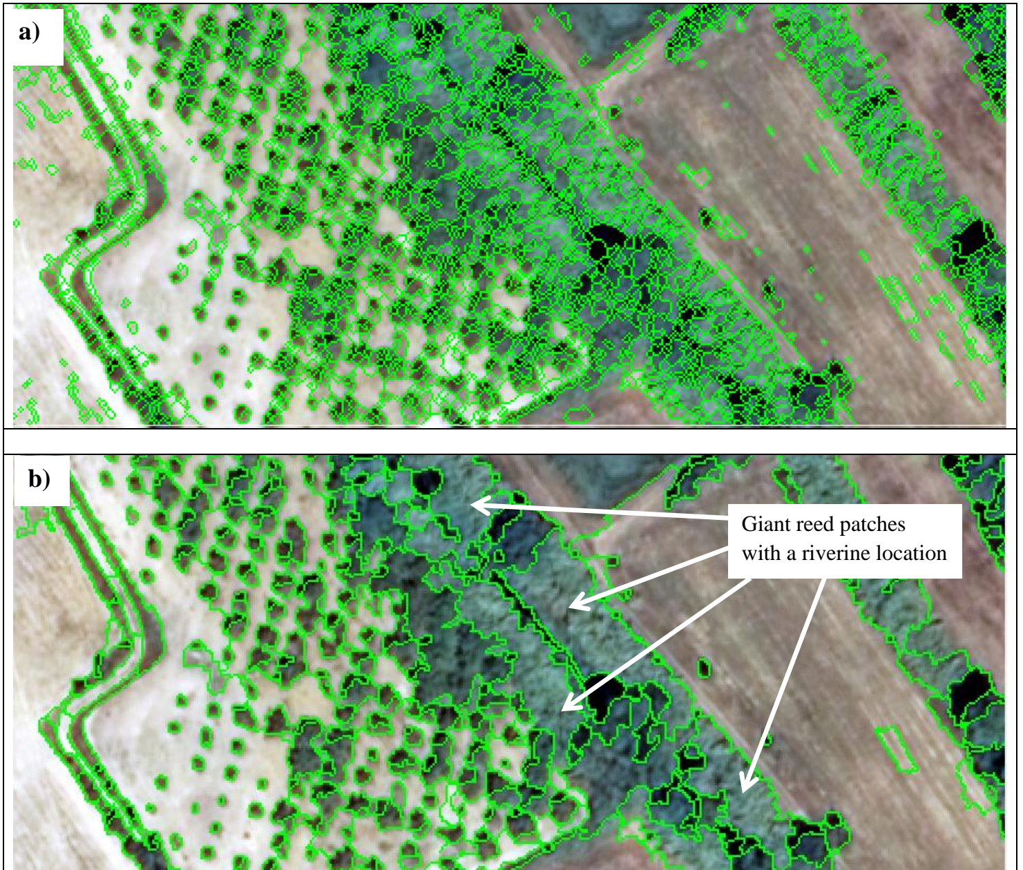
Figure 1 – Partial output of the airborne multispectral image Set07 in true-color composition (red, green and blue bands), a) initial segmentation output with a scale level of 40.0 b) segmentation output with a merged lambda value of 90.0 to eliminate the over-segmentation.
