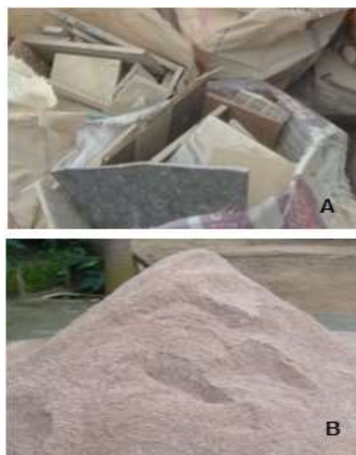
Fig 1: Recycled ceramic tile before (a) and after (b) crushing
