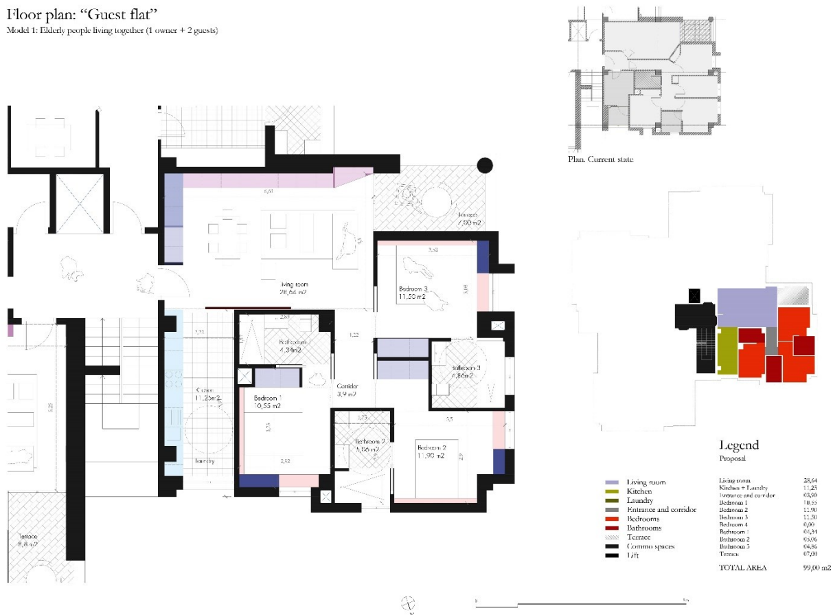
Figure 11. Model 1 (Host flat or Guest-flat). Proposal for the transformation of the house for co-aging.
