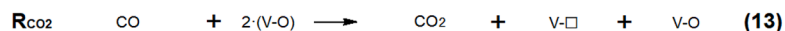
Scheme 1. Proposed detailed mechanism of the propane ODH. adapted from Ternero-Hidalgo et al., 2021
