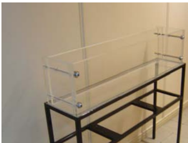
Figure 1- Track where animals walked, (Perspex 120cm length, 12cm width, and 15cm height)
