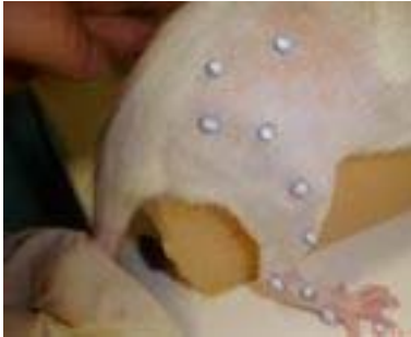
Figure 6 - Reflective markers with 2mm diameter were attached to the right hindlimb at bony prominences: (1) tip of fourth finger, (2) head of fifth metatarsal, (3) lateral malleolus, (4) lateral knee joint, (5) trochanter major, (6) anterior superior iliac spine, and (7) ischial tuberosity and three non-collinear markers.
