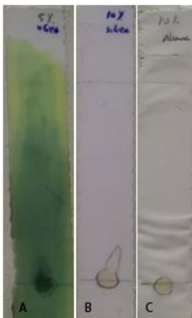
Fig. 15 - TLC of the methanolic extract (MF2) using different sheets. A - Precoated silica TLC sheet using dichloromethane (5% v/v) and methanol (95% v/v) as eluent B - Precoated silica TLC sheet, using dichloromethane (10% v/v) and methanol (90% v/v) as eluent. C - Precoated alumina TLC sheet, using dichloromethane (10% v/v) and methanol (90% v/v) as eluent.
