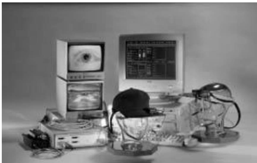
Fig. 150 - Sistemas de tracking Polhemus FASTrak and VISIONTrak (Carlson 2003, section 17 ).
