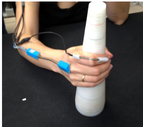
Figure 3. Hand instrumented with electronic goniometers to measure the posture while grasping the cone.
