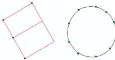
Figure 5 - Example of a roof of a house and of a well measured for the quality control of the laser data
