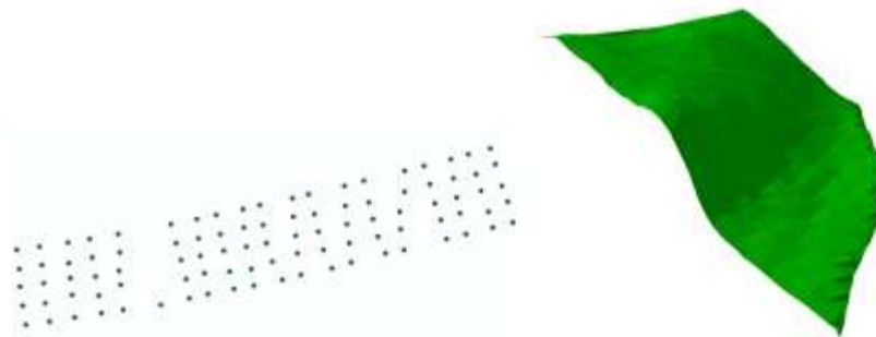
Figure 6 - DTM on flat surfaces (road and field) for the quality control of the laser data
