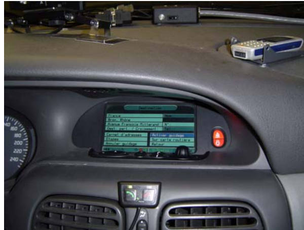
Figure 18. Guidance system display and below the two interface buttons for the mobile phone
