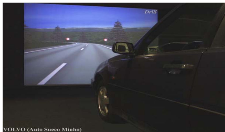
Figure 24. Image of the simulator room with the car and the screen for the projection of the road scenario
