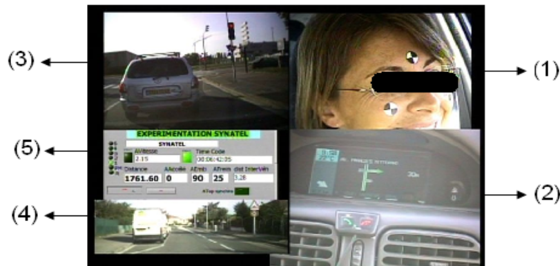
Figure 16. Combination of all the images from the cameras and also from the program that gathered the dynamic data of the vehicle
