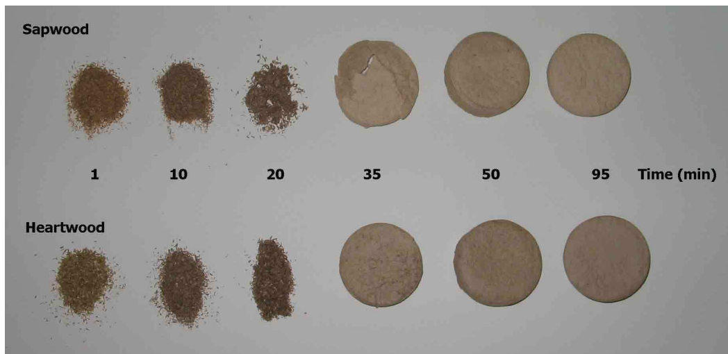
Figure 8. Samples of 20-40 mesh fractions of sapwood and heartwood of E. globulus after delignification with different times (1 to 95 min).
