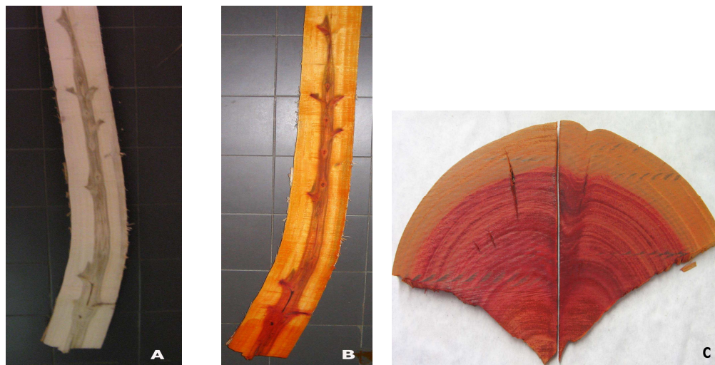
Figure 3. E. globulus wood: A – log showing sapwood and heartwood areas; B – the same log after application of methyl orange (used to increase distinction between both areas); C – transversal section of one wood disc after methyl orange application.
