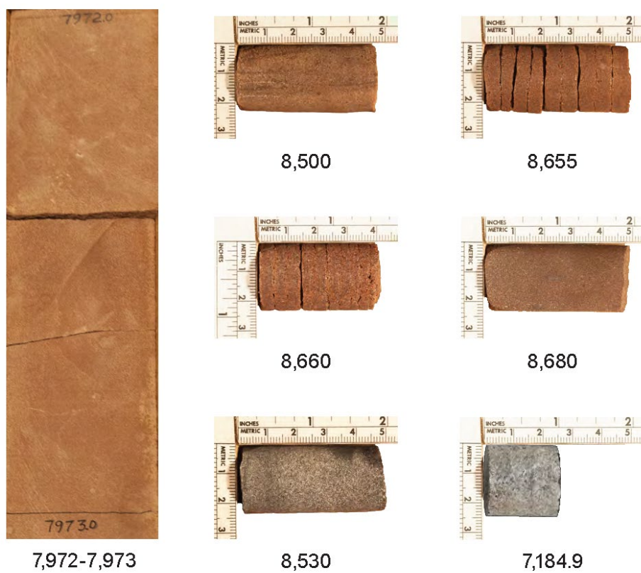
Figure 5: Photographs of Wabash #1 well Mt. Simon Sandstone full diameter (3.5 inch) core sample from 7,972-7,973 and rotary sidewall core samples (1-inch diameter) from the Wabash #1 well and Verification #2 well. Samples depths (ft) 8,500; 8,655; 8,660; 8,680 are sandstone and were disaggregated for detrital zircon extraction and U/Pb dating. Sample depths (ft) 8,530 is a basalt from Wabash #1 well and 7,184.9 is a gabbro from Verification #2 were prepared for Ar/Ar dating.
