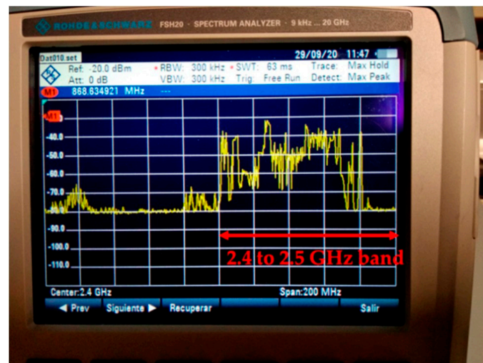
Figure 2. RF interference measurements within the factory workshop at the 2.4 GHz band.
