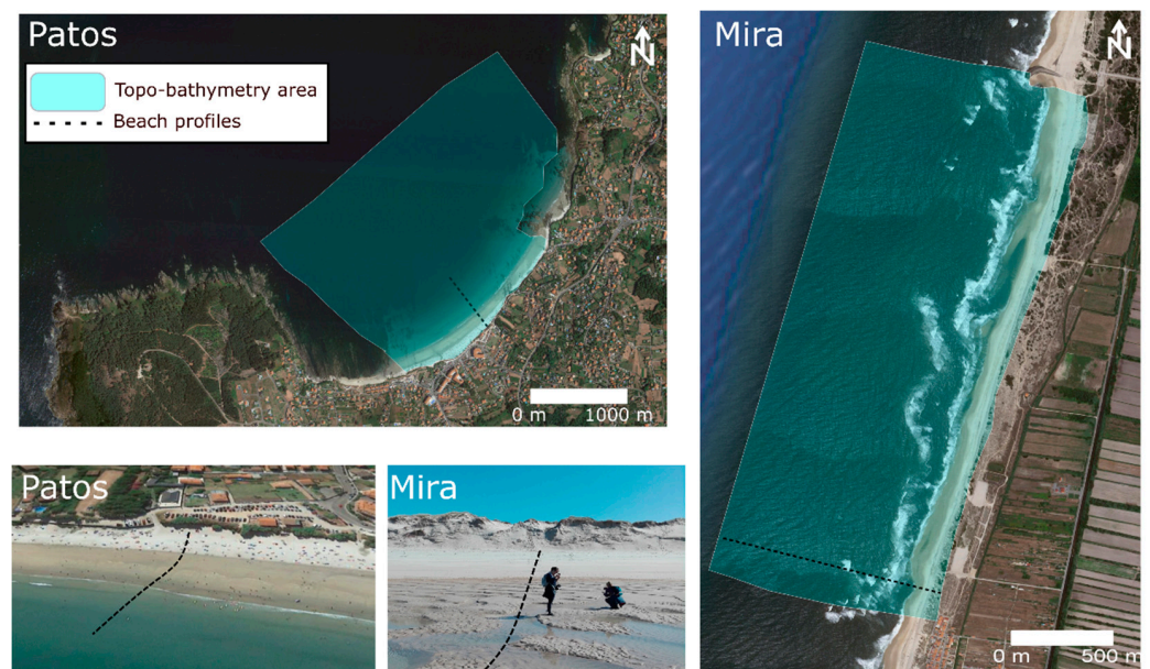
Figure 2. Images showing the RTK_DGPS beach profiles (black dashed lines) and topo bathymetric survey areas (marked in green) in Patos (left) and Mira (right) beaches.
