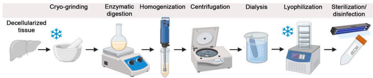
Fig. 2. A schematic presentation of typical steps in the dECM solubilization to make the material ready for the bioink or bioresin formulation.
