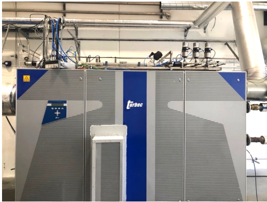
FIGURE 5: TURBEC T100 UNIT WITH MODIFIED COMBUSTOR AND FUEL TRAIN FOR FLEXIBLE FUEL OPERATION [25].
