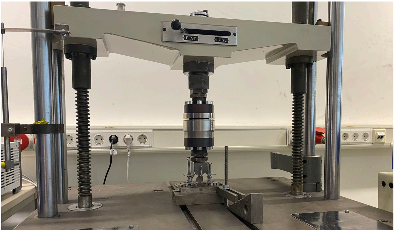
Figure 2. Test bench when determining the splitting tensile strength.
