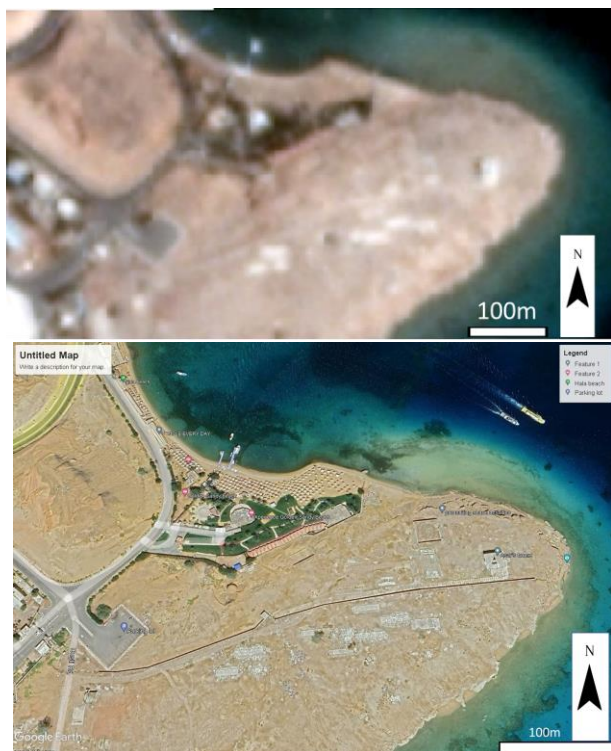
Figure 9. Compare the performance of Geoeye-1 (3 m) in the upper photo with that of Google Earth Pro in the lower one.
