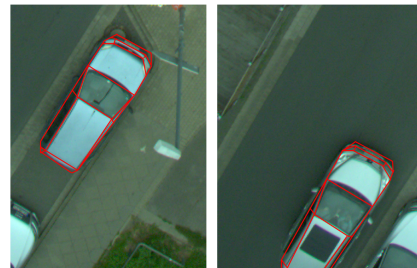
Figure 3. Qualitative results of V_{L1} on two UAV test images. The backprojected shapes of the reconstructed vehicles are represented by red wireframes.
