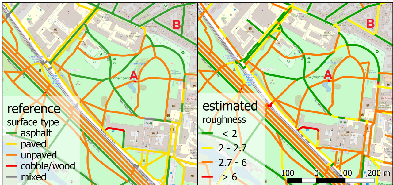
Figure 6. To give an example of the results, way segments in and around the university park are colored by their surface type (left) and by the estimated roughness value (right). They are ordered by smoothness and colored from green (asphalt - smooth) to red (cobblestone/wood planks - rough). For an easy comparison the estimated roughness values are also grouped into four related classes. (base map and data from OpenStreetMap)
