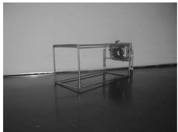
Fig. 2 Waterproof casing attached to stainless steel structure
