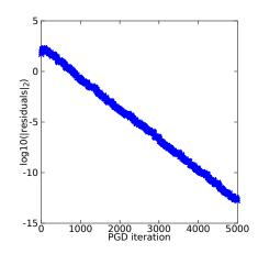
Figure 3: The evolution for the residuals for 5000 steps of PGD by using (25) for a matrix of size  $5832 \times 5832$ . The CPU time was of 4070.55 seconds.
