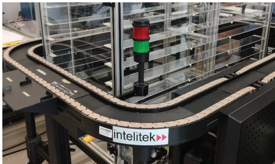
Figure 9: Intelitek pallet conveyor (Martins et al., 2019).
