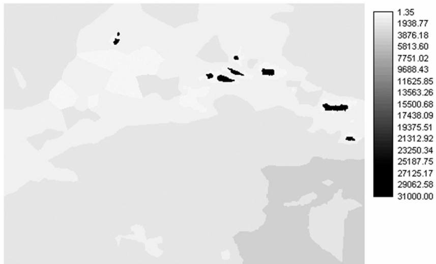
Fig. 7. Friction surface comprising different types of weighted data: bathymetry, land, number of individuals caught and oil barrels obtained. The scale represents pixel weight values.
