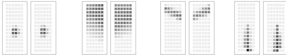
(c) Tactile images taken at the grasping position (white = 0, black = max) for the left and right tactile sensor
