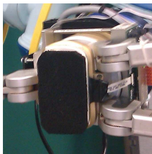
Figure 5: Low density conductive foam (RS-55-066) used on the experimental tactile sensors for the Tombatossals Robot in the Robotic Intelligence Lab at UJI
