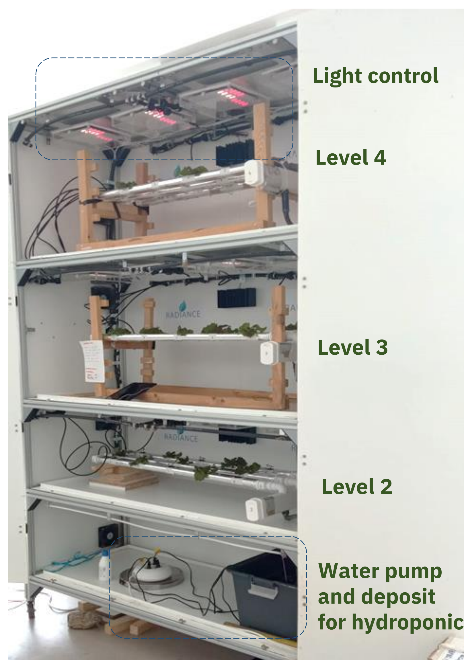
Figure 1- Hydroponic chamber consisting of 3 levels, light control, temperature and humidity monitoring, capacity for 45 plants and tank/pump.
