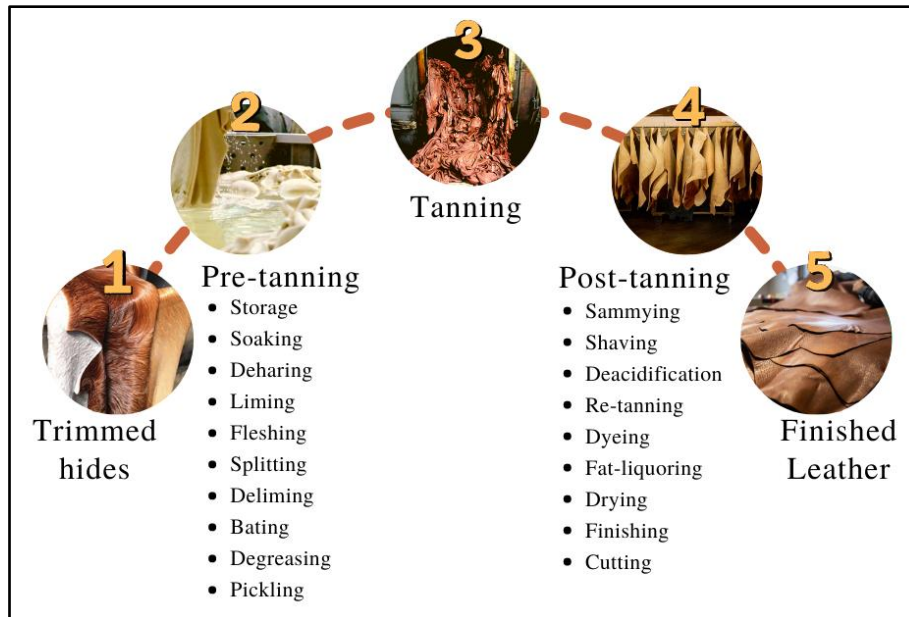
Figure 4. Generic leather processing diagram. Source: Own design.
