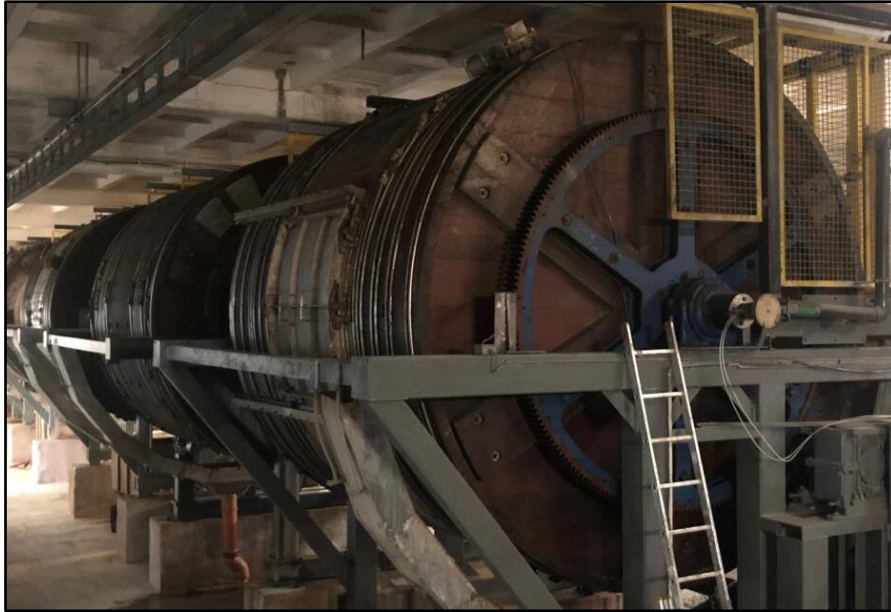
Figure 5. Rotary drums are employed in the soaking, liming, deliming, tanning, and dyeing stages. Source: Tannery Projects (2022).
