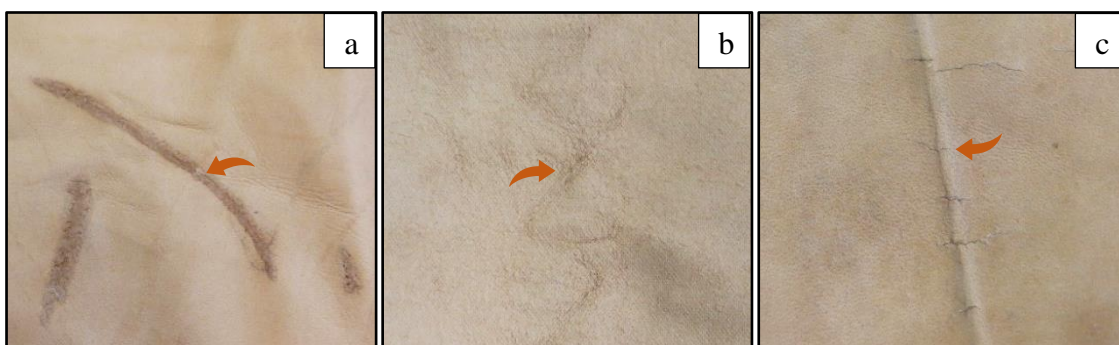
Figure 6. Defects of (a) scars, (b) material loss, and (c) cracks found in leather, each marked with an arrow. Source: Photos taken by the author.
