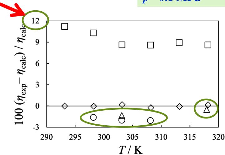
Deviations of the viscosity results for  $[P_{6,6,6,14}][dca]$ , obtained by Pereiro et al.,<sup>33</sup> □, and in the present work using: the vibrating wire technique, ◇ (nominal values from Table 6); an Ubbelohde capillary, ○, and an Ubbelohde microcapillary, △, from the correlation eq 10 with the parameters of Table 5.
