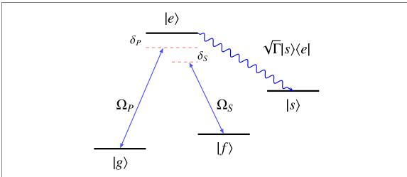
Figure 1. Schematic energy level structure for the lambda system modulated by detuned AC-driving fields with respective Rabi frequency  $\Omega_P$  and  $\Omega_S$ . The scheme includes a sink state  $|s\rangle$ , coupled to the excited state  $|e\rangle$  of the system, as a means to induce a loss mechanism at rate Γ.
