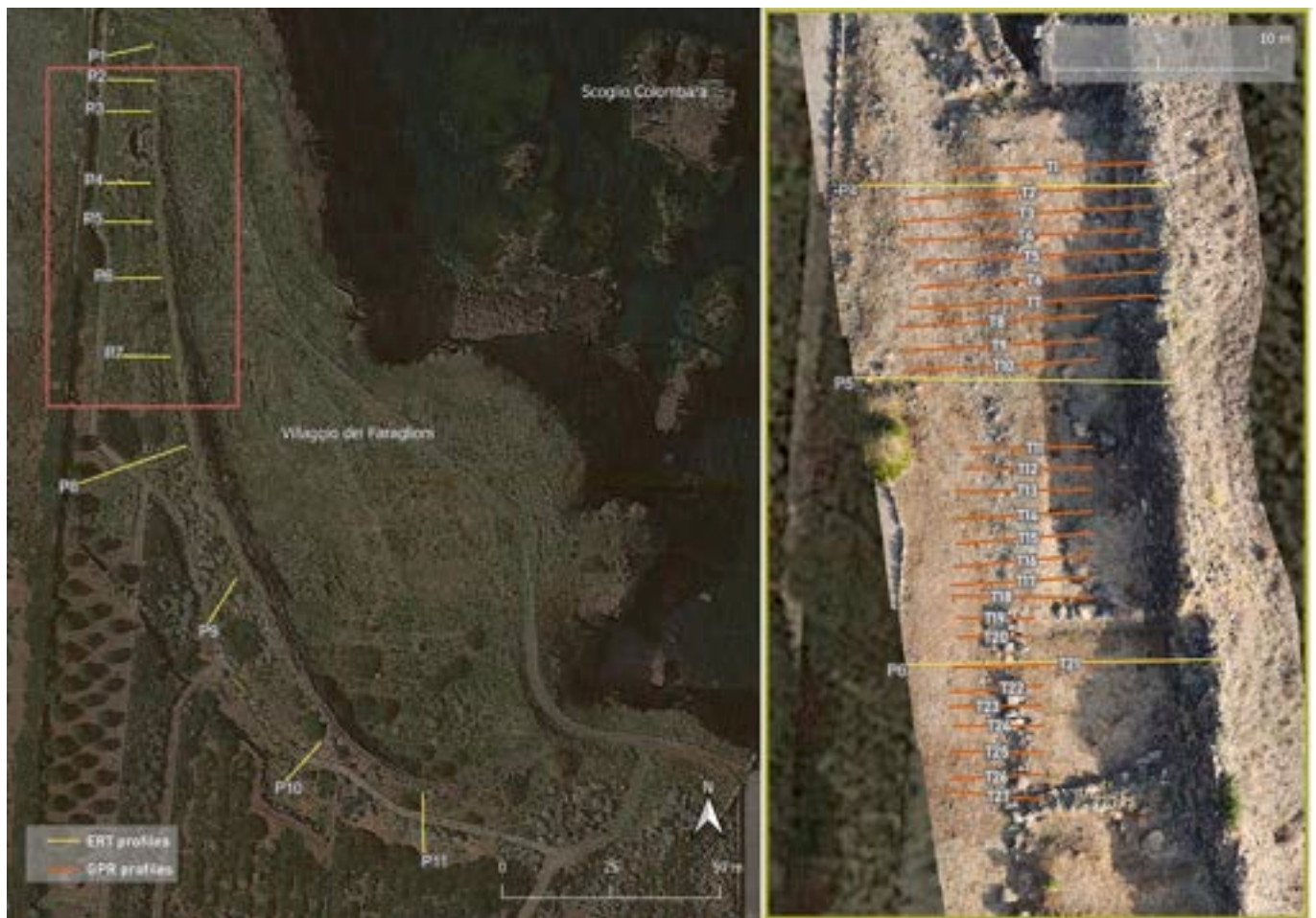
Fig. 9. Left panel) ERT profiles (solid yellow lines). Right panel b) GPR profiles (solid red lines) acquired during the geophysical survey. The red box in panel left, indicates the position of the subset area in which GPR profiles were performed. Both acquisition layouts are superimposed to a high-resolution orthographic picture of the investigated area (Russolillo et al., 2022). Some profiles from different investigation techniques overlap (ex. P4 with T2, P5 with T10 and P6 with T21). (For interpretation of the references to colour in this figure legend, the reader is referred to the web version of this article.)
