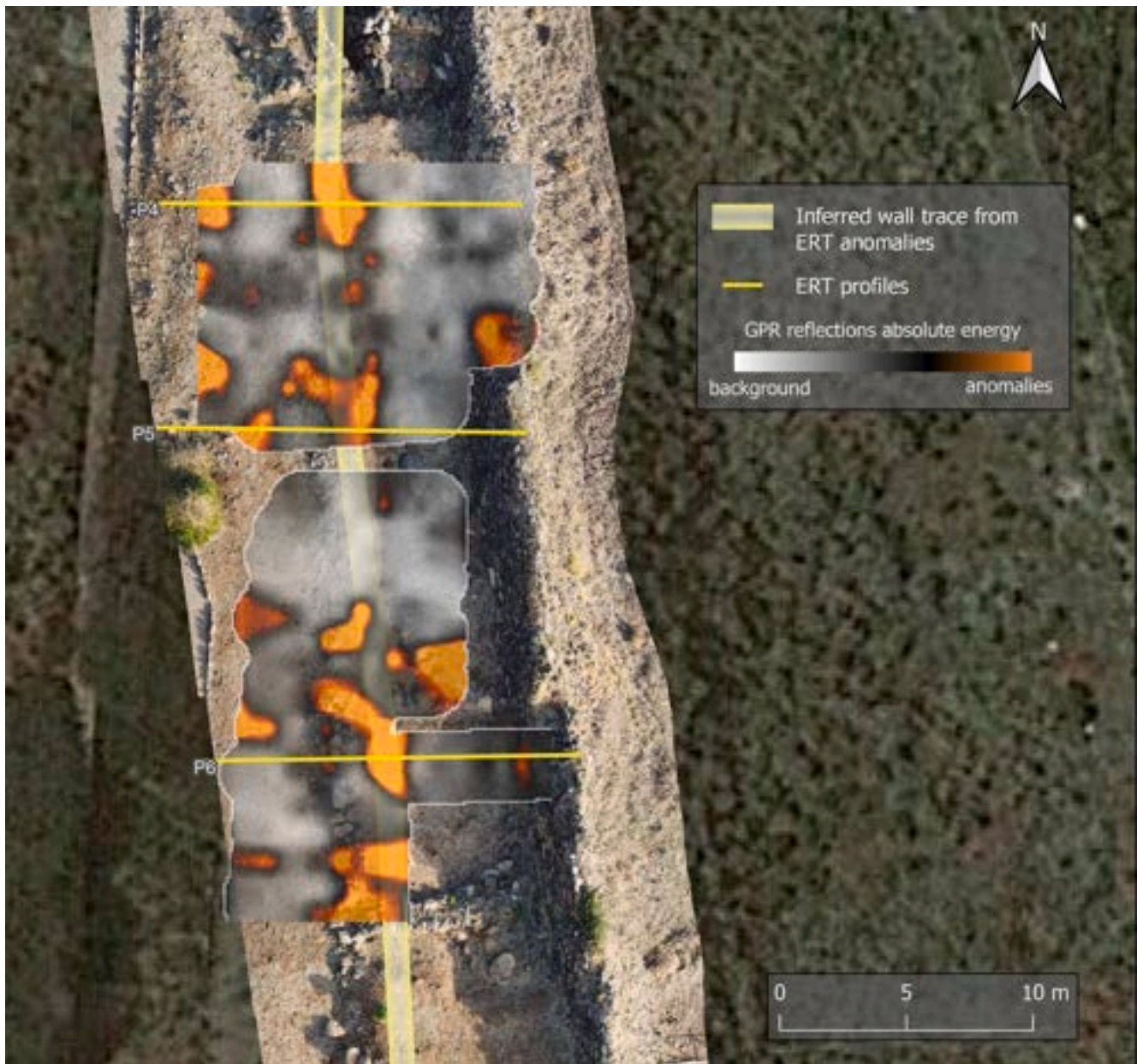
Fig. 17. Time-slice analysis between 0.6 and 0.8 m that highlight a clear alignment of electromagnetic reflection, which also aligns with the inferred wall trace interpreted from ERT anomalies.
