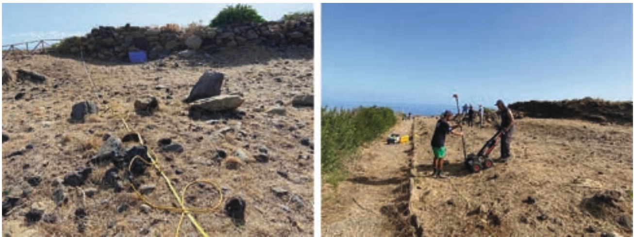
Fig. 8. Left) example of an ERT acquisition in the northern sector of the survey area, right) operators while performing the GPR survey in the southern sector.
