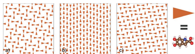
Fig. 5 The ordered structures of DHICA obtained by MC calculations: (a) open lattice, (b) brick wall, and (c) ladder phases.
