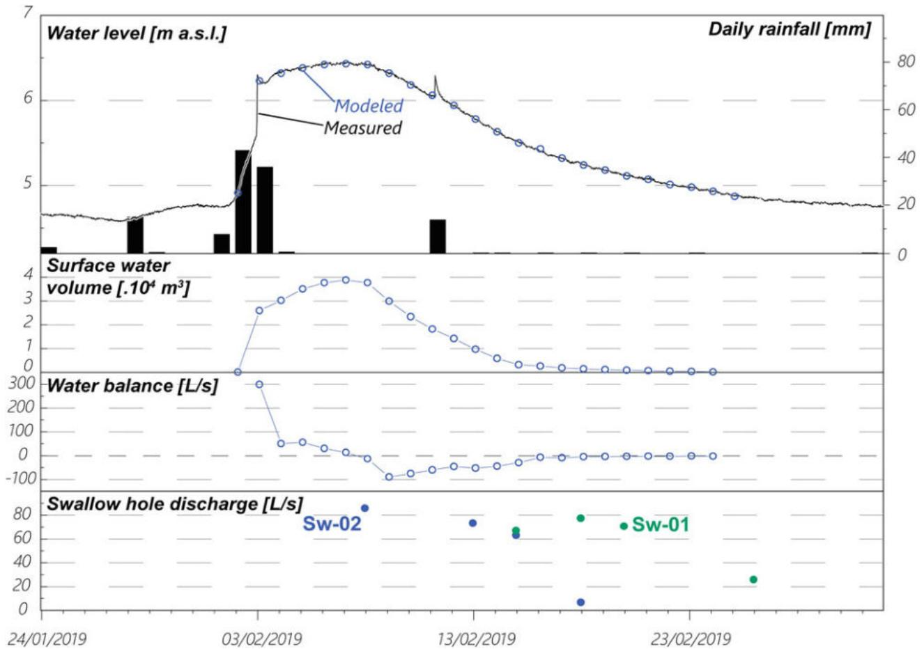
**Fig. 6** Water level measured in the S20 piezometer and daily rainfall data from Gorizia Italy (provided by ARPA-OSMER) during event 2. The water level allows the calculation of the surface water volume and consequently the daily mean water balance. Discharge values (in situ measurements) of both swallow holes are plotted in the lower graphic
