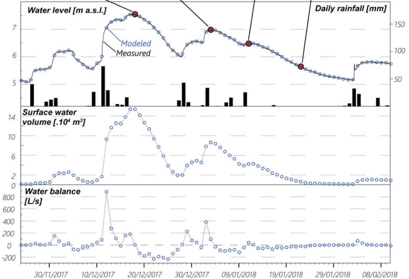
**Fig. 5** Water level measured in the S20 piezometer and daily rainfall data from Gorizia Italy (provided by ARPA-OSMER) during event 1. Photographs illustrate the situation in the Sw-02 at different levels. The water level allows the calculation of the surface water volume (middle graphic) and consequently the daily mean water balance (lower graphic)
