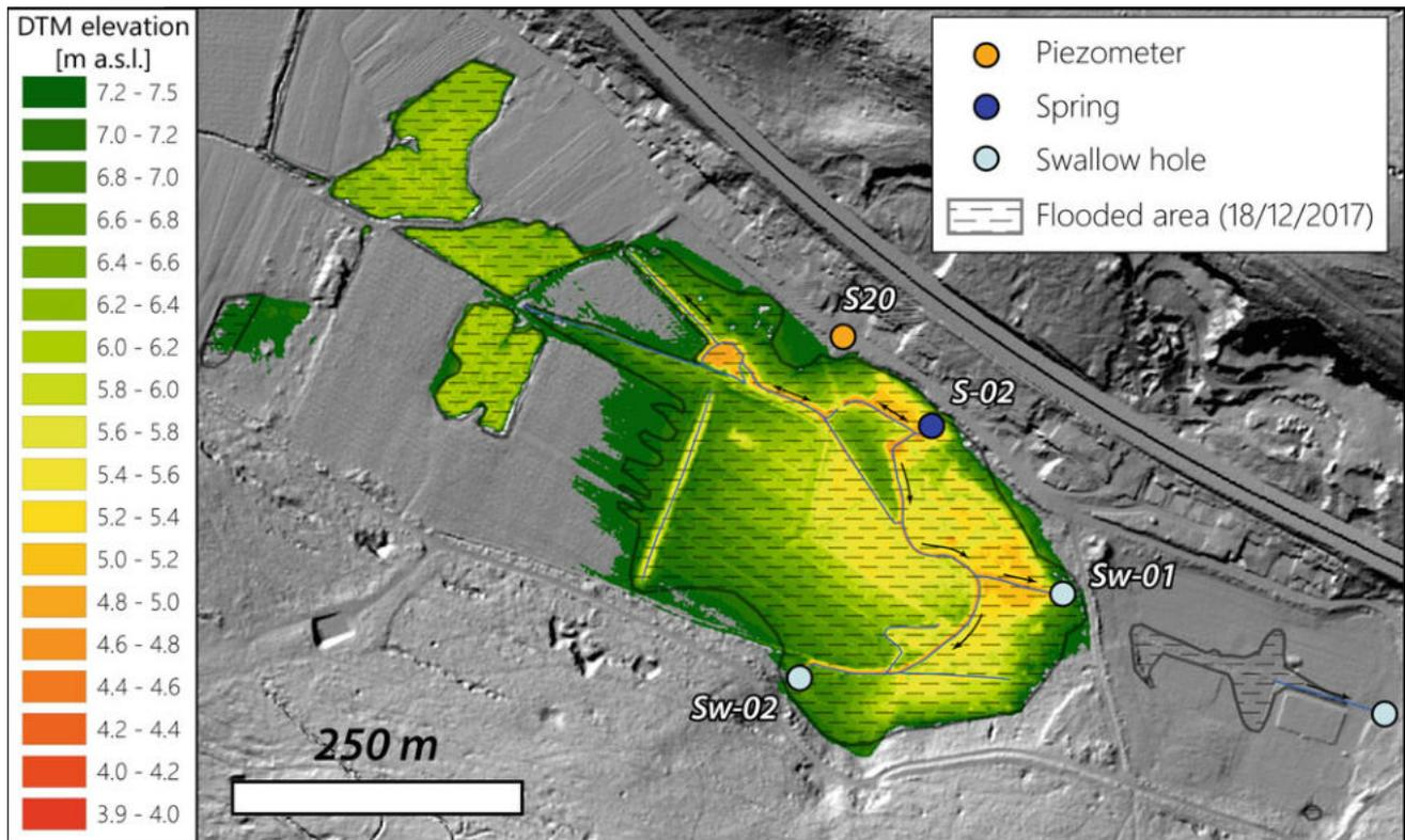
**Fig. 3** DTM of the Mucille depression. The flooded area at the peak of event 1 (18/12/2017) coincides with the 7.5 m a.s.l. elevation. The surface water volumes calculated with DTM allow the modeling of the water table elevation as function of the surface water volume
