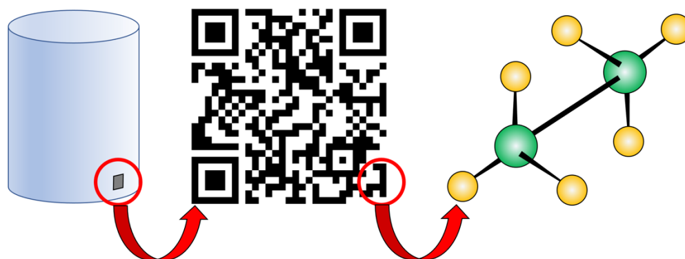
Figure 1. Example of a multi-level tagging feature that is composed of an ouverte QR code and of a chemical fingerprint (the static QR code redirects to A. Sola's ORCID page, https://orcid.org/0000-0002-8649-9388 (accessed on 22 December 2021); the image is only for illustrative purposes, and the chemical structure shows a mock compound).
