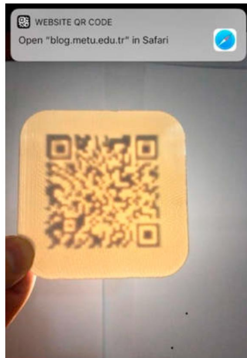
Figure 4. Example of scanning a QR code with background light. Reproduced from Reference [24], Gültekin et al. Procedia Manuf. 2019 , 39 , 519–525, https://doi:10.1016/j.promfg.2020.01.411 , under the terms of the CC BY-NC-ND license.
