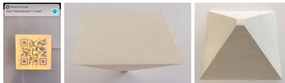
Figure 5. Example of scanning a QR code embedded into a 3D object. Reproduced from Reference [24], Gültekin et al., Procedia Manuf. 2019 , 39 , 519–525, https://doi:10.1016/j.promfg.2020.01.411 , under the terms of the CC BY-NC-ND license.
