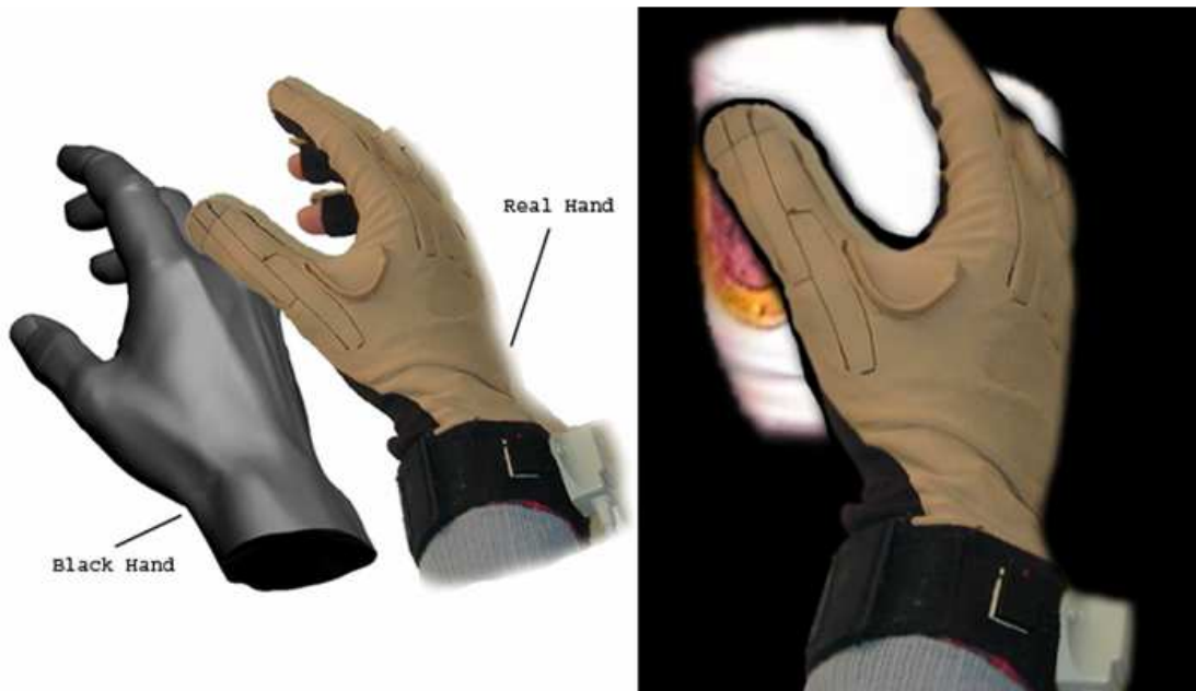
Figure 4: (Left) Black Hand and real hand; (right) the effect achieved after applying the “Black Hand” paradigm.
