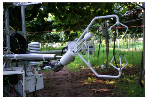
Fig. 2. (Top) Vertical mast hosting three aligned eddy covariance systems: above the net, between net and the canopy, and below the canopy. (Bottom) Detail of the below-canopy system (sonic anemometer, infrared gas analyzer, net radiometer, thermo-hygrometer).
