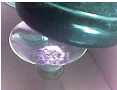
Fig. 1 Irradiation with a mercury UV lamp of 60 W maintaining an air flow of 6 l/min through the photocatalyst for 48 h
