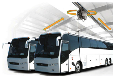
FIGURE 6. Charging reels for flexible charging cabling in depot charging.
