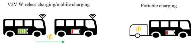
FIGURE 18. E-bus alternative charging system.
