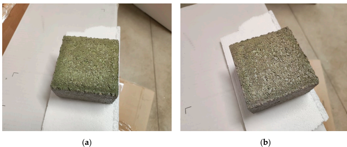
Figure 2. (a) The partially immersed “Wet Block”; (b) the “Dry Block”.
