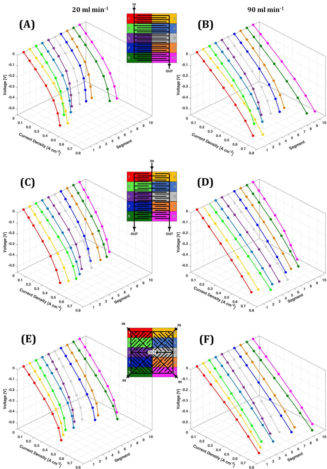
**Figure 8.** Local polarization curves with (A,B) Interdigitated, (C,D) Two Outlets and (E,F) Four Inlets geometries at 20 mL min<sup>-1</sup> (A,C,E) and 90 mL min<sup>-1</sup> (B,D,F). Miniatures: schematic representation of the segmented flow fields.
