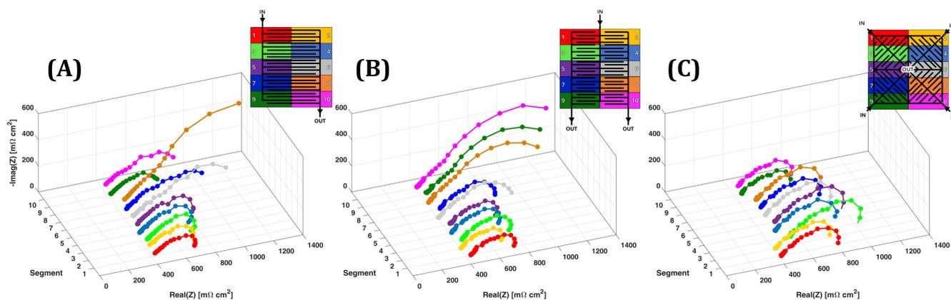
**Figure 9.** Nyquist plots of local electrochemical impedance spectra at  $0.1 \text{ A cm}^{-2}$  and  $20 \text{ mL min}^{-1}$  with the (A) Interdigitated, (B) Two Outlets and (C) Four Inlets flow fields. Miniatures: schematic representation of the segmented flow fields.
