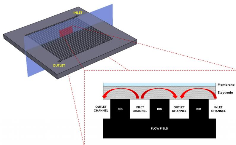
**Figure 1.** Schematic representation of under-the-rib fluxes with Interdigitated flow field geometry.
