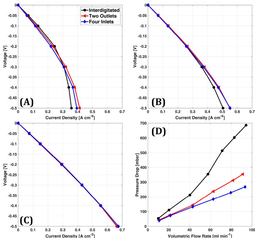
**Figure 7.** Polarization curves with the different flow field geometries at (A) 20 mL min<sup>-1</sup>, (B) 40 mL min<sup>-1</sup> and (C) 90 mL min<sup>-1</sup>. (D) Pressure drops through the cell at different volumetric flow rates.
