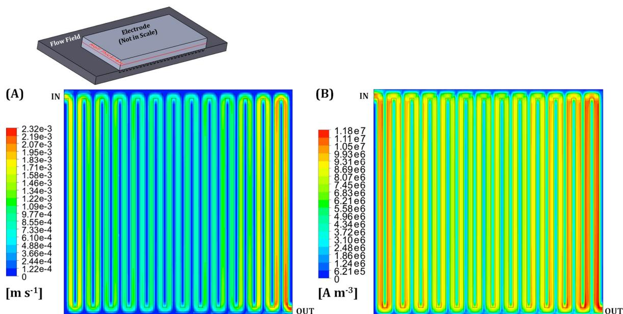
**Figure 4.** Velocity magnitude (A) and reaction rate (B) with the Interdigitated geometry at  $0.15 \text{ A cm}^{-2}$  and  $20 \text{ mL min}^{-1}$  on a plane at half electrode thickness. Miniature: position of the plane at half electrode thickness (red line).
