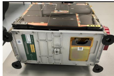
Figure 11 (left). Deep Space Deployer and Life Support Interface Board Figure 12 (right). Milani CubeSat Interface Board (interfacing the CubeSat with the DSD pusher plate)
