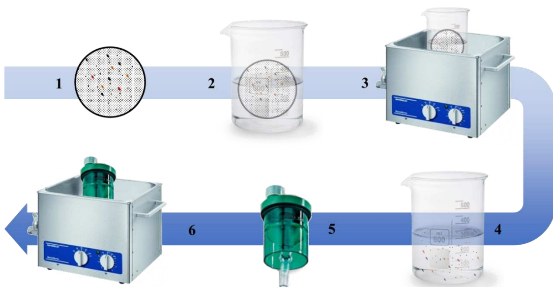
Figure 75. Procedure steps for suspension production. 1) loaded filter; 2) filter immersion in pure water; 3) ultrasonic bath for particles detachment and suspension; 4) suspension; 5) nebuliser tank filling; 6) aerosolization in ultrasonic bath.
