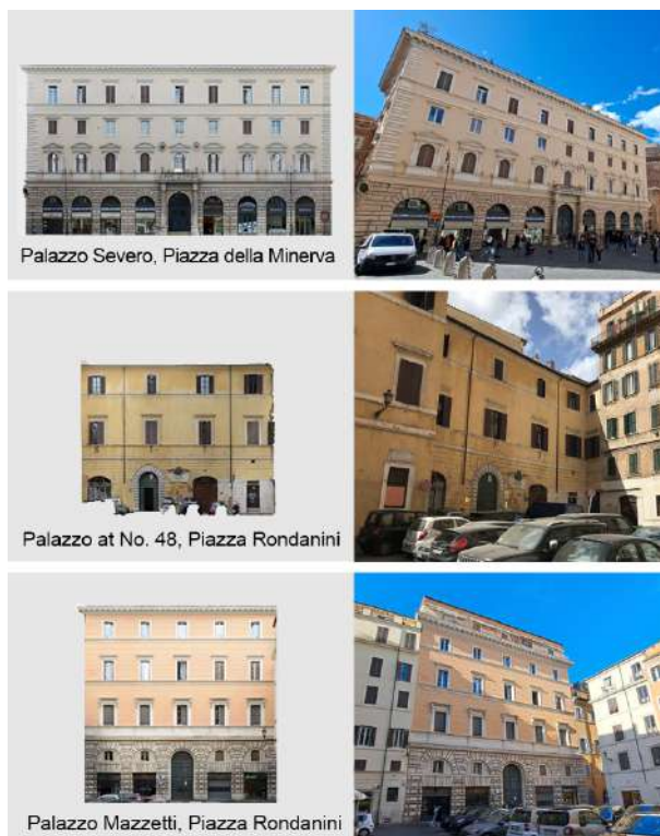
Figure 6: Facades orthoimages (left) and photographs of the urban context (right) in which the selected palaces are located.
