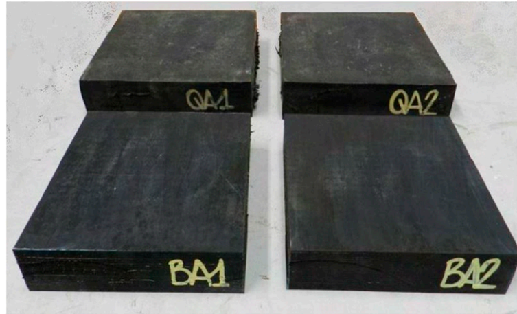
Figure 4. Photo of the isolators. Note that the names of the specimens in this paper were shortened from QA1, QA2, BA1, and BA2 to Q1, Q2, B1, and B2, respectively, for brevity.
