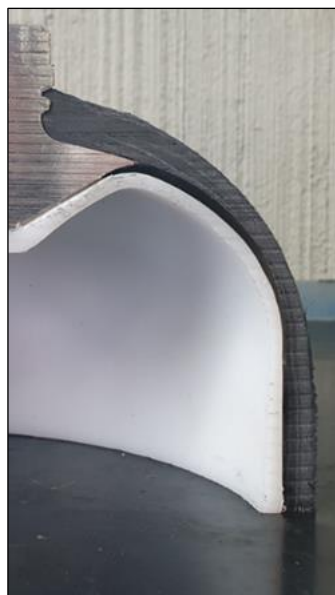
Figure 8. Section of the cured high-pressure storage tank.
