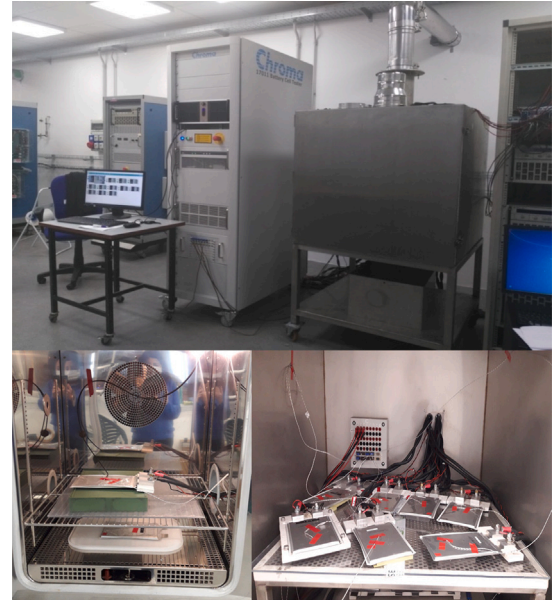
Fig. 11. Working station used to perform the aging test on lithium-ion cells.
