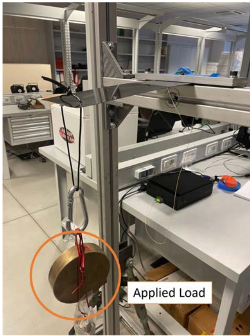
Fig. 7. Experimental set-up for mechanical characterization using calibrated loads.
