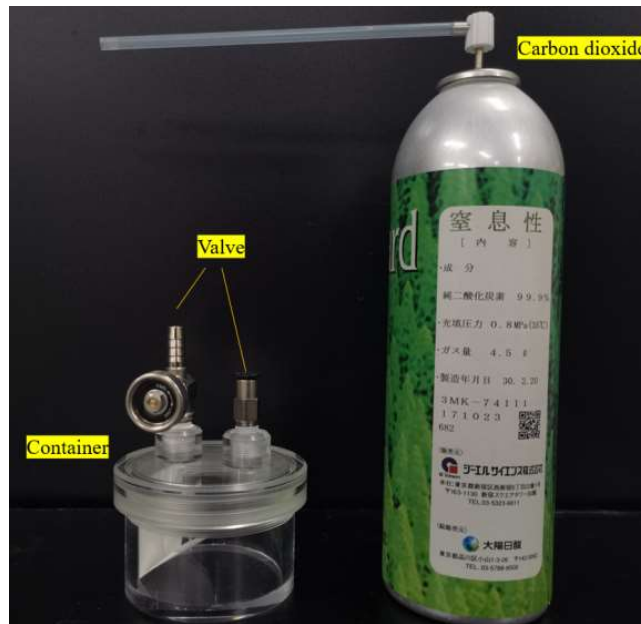
Figure 2-2 Container for accelerated carbonation test
